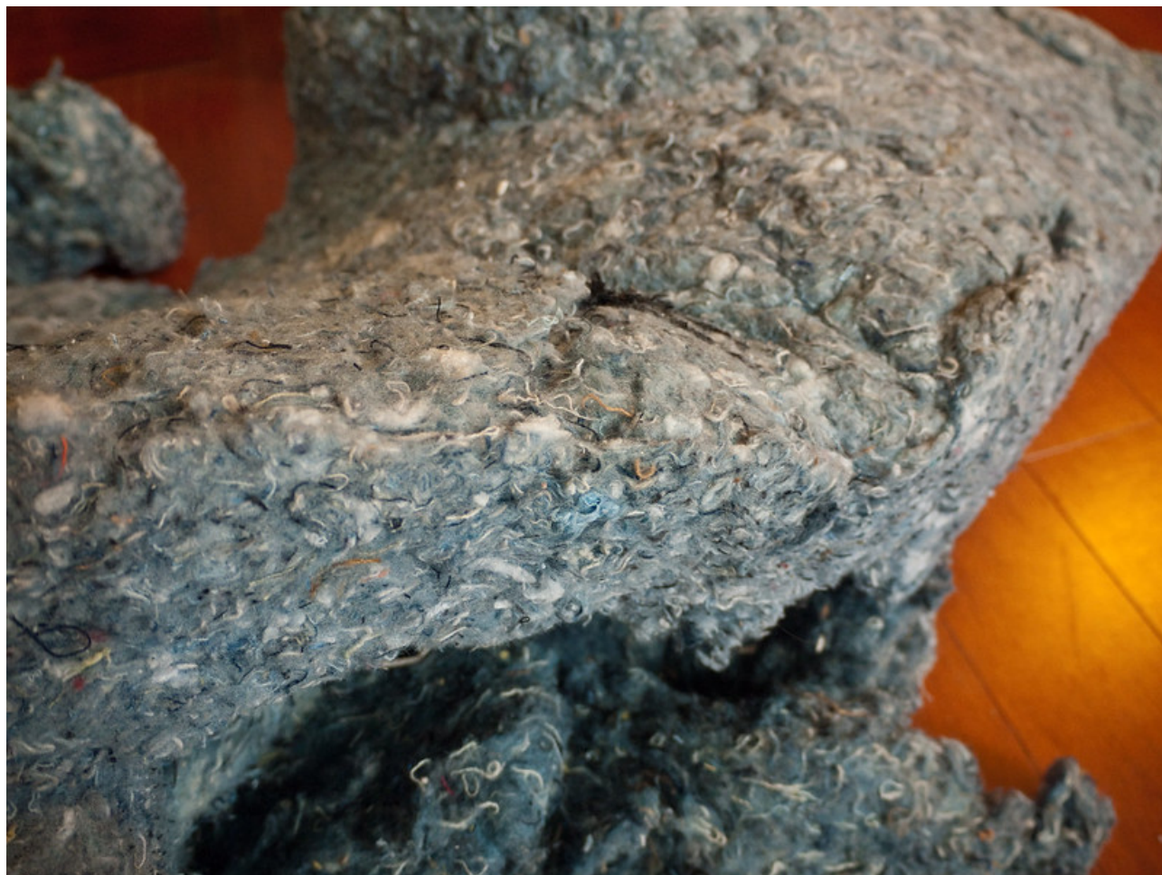
Figure 5.3.2 – Insulation material made from recycled cotton jeans
