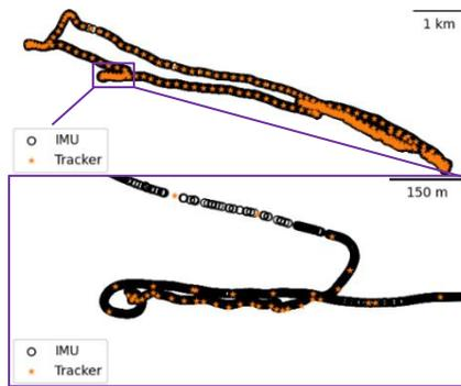
Figure 1. Comparison of the lat-lon points obtained by the two devices fixed at the vessel
