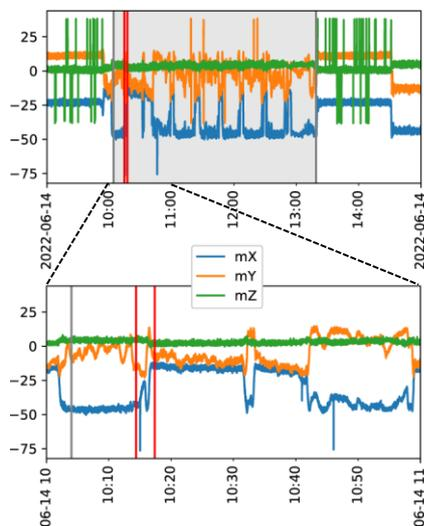
Figure 2. Three-component magnetometer data. Red lines indicate the presence of the aRFID onboard.
