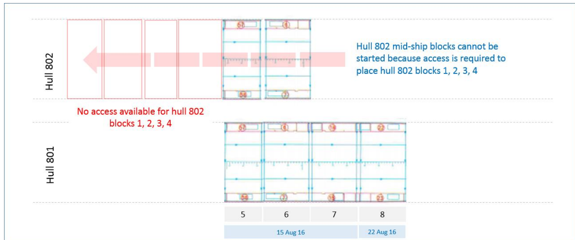
figure 3-14 hull 802 midship blocks obstruct 802 stern blocks
