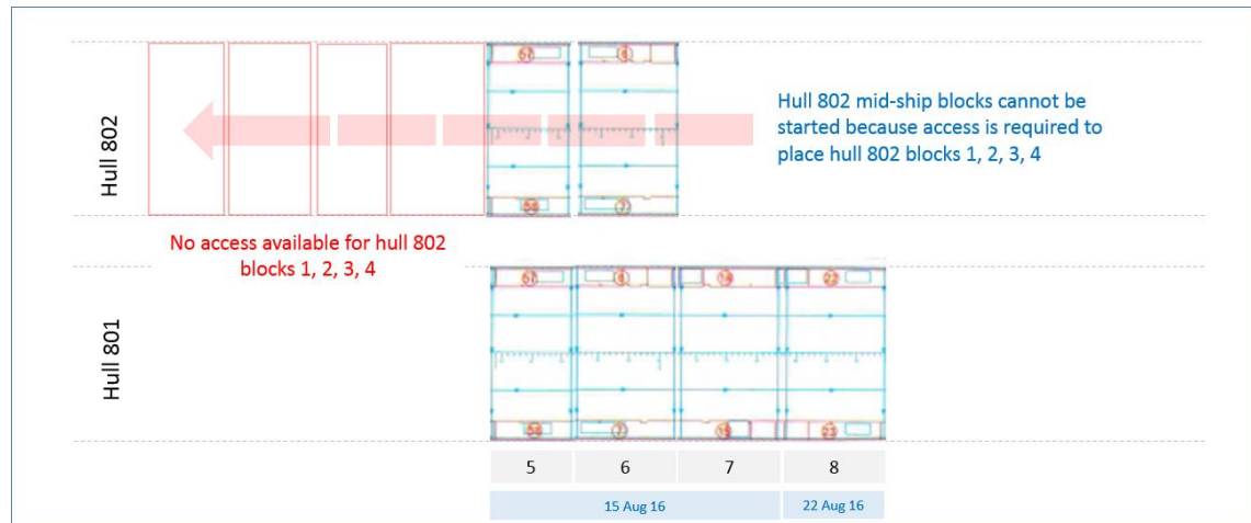
figure 3-14 hull 802 midship blocks obstruct 802 stern blocks
