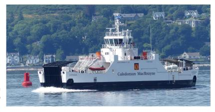
Our vessel engineers were responsible for introducing the world's first diesel-electric hybrid ferries, MV Hallaig (2012), MV Lochinvar (2014) and MV Catriona (2016). This technology enables these three vessels to operate on the batteries for 30% of each working day. The batteries are charged using shore power connections from the grid.
